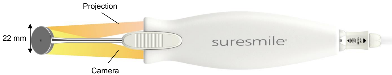
Figure 2: orascanner 2 Light Path
