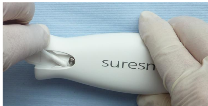
Figure 8: Cleaning the orascanner mirror Mount
