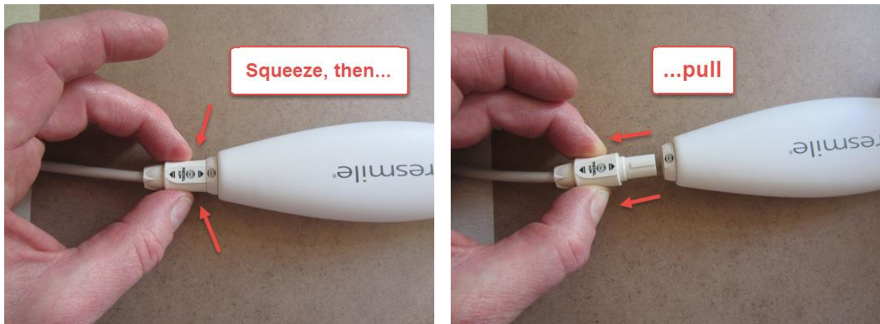
Figure 9: Removing the USB Cable from the orascanner 2
